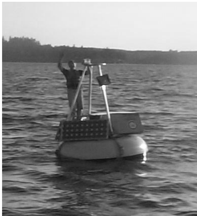
Figure 1. The Oceanic Remote Chemical/Optical Analyzer (ORCA).
