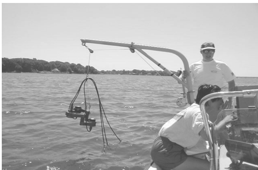
Figure 1. Technicians measuring underwater light spectra and light attenuation at the Rhode River CISNet Site.
