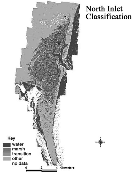
Figure 1. Neural network classification of North Inlet intertidal marshland and open water based on an ADAR image with a 60 cm spatial resolution.
