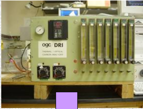
Original OGC/DRI Thermal Optical Analyzer (1986)
