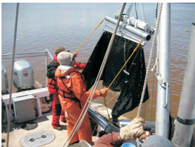
G. Peterson (left) and J. Hoffman (center) retrieve a tucker trawl sample from aboard the R/V Prairie Sounder . The trawl is used to collect fish larvae in the water column. The instrument mounted to the top bar of the trawl measures water conductivity, temperature, and depth and transmits the data in real-time to the research vessel.
