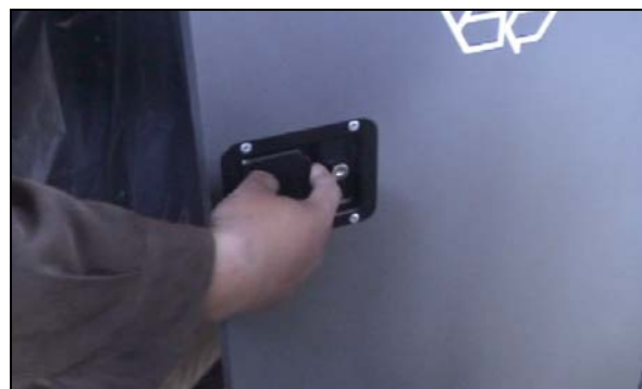
(36) New design to solve key and handle breakage problems
