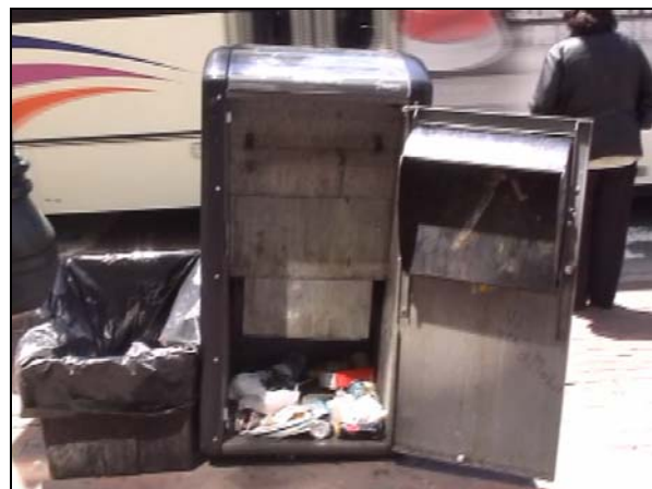
(11) Compaction ram stuck in down position, unit not stable and leaning to the right
