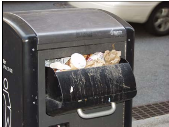
(31) A trash compactor that is full and will not compact trash
