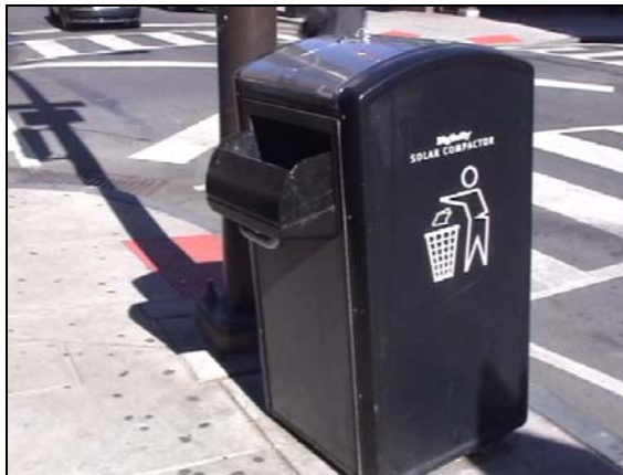
(27) A door that will not automatically shut because the unit is not level
