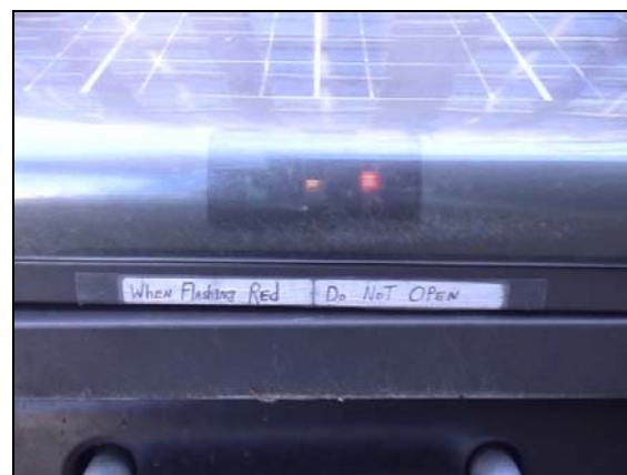
(30) Lights indicate the unit is out of service. Note the hand made and taped on sign
