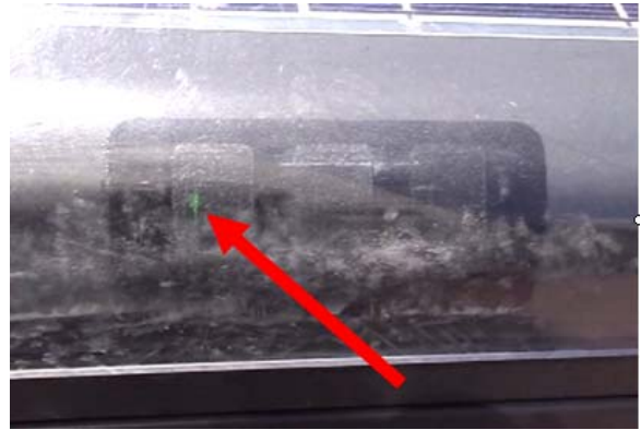
(12) Compactor unit is not working yet green light is on indicating "system normal"
