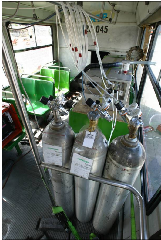
Inside view of retrofitted bus during emissions measurement, showing trace gas containers.
