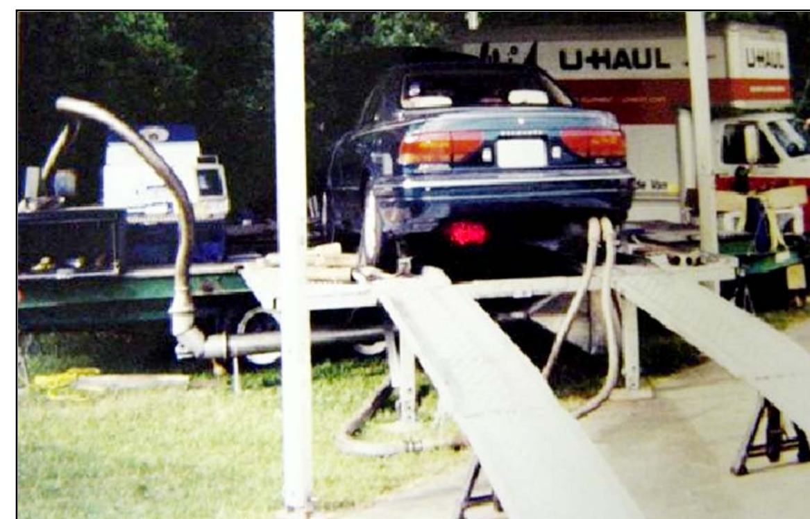
NERL Portable Dynamometer used in Kansas City Light-Duty Vehicle Emission Study and the Gas/Diesel Split Study.
