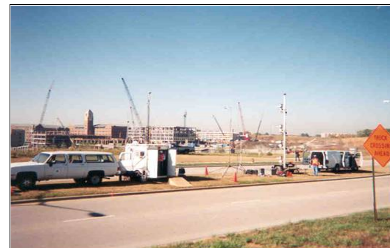
Test set-up for Kansas City construction dust study using both continuous (left) and manual (right) sampling arrays.
