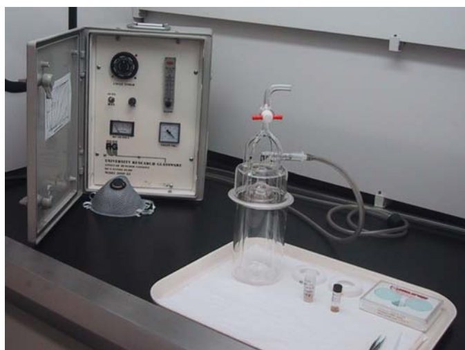
Figure 3-4. "Puffer" apparatus used to prepare filter samples of bulk dusts and powders. The side arm below the shut-off valve is connected to a vacuum pump.
