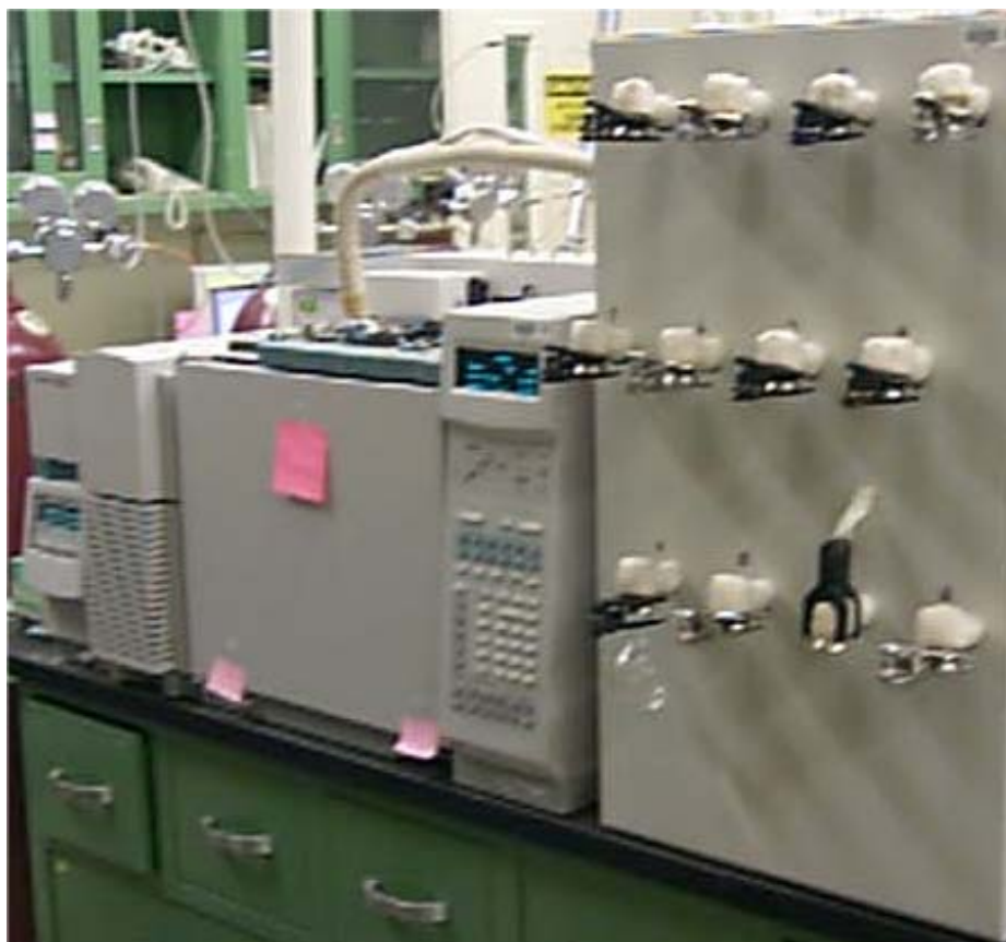
Commercial vacuum distiller configured with Agilent 5973/6890 GC/MS
