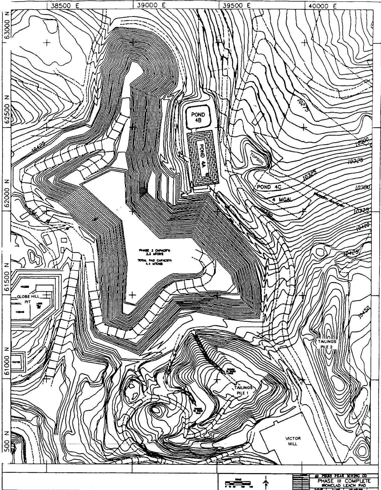
Figure 4-3. Planned Final Configuration of Ironclad Heap
