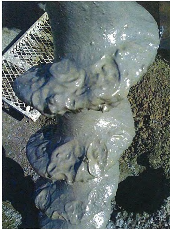
Photograph 7 – Soft saturated clay found in Borehole LEC-7 (looking northeast)
