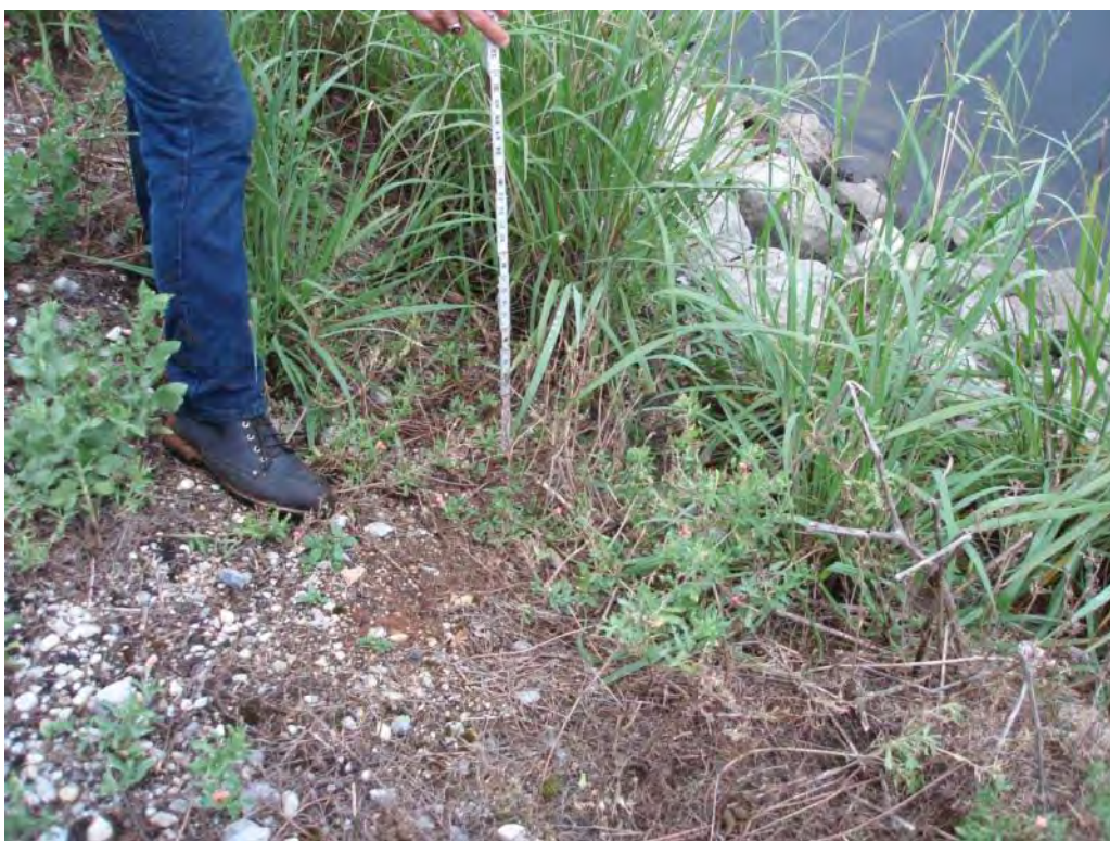
Photo No. 108: #2/#3 Bottom Ash Pond – West embankment interior slope. Looking at surface erosion and possible localized settlement.
