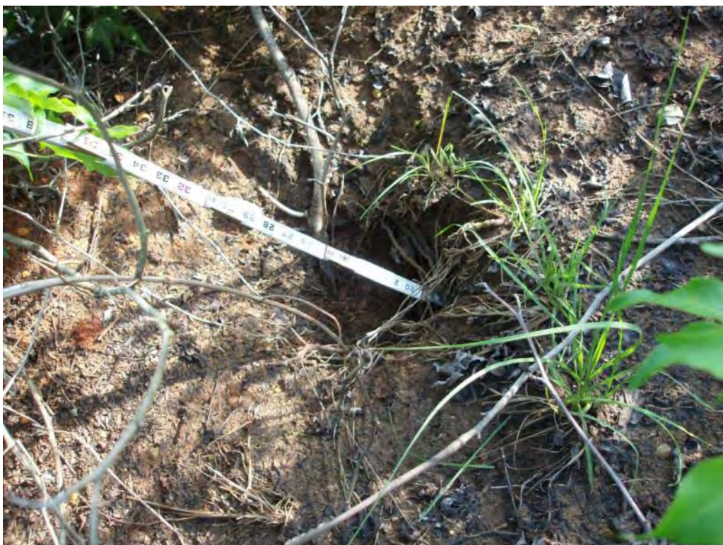
Photo No. 154: Scrubber Waste Pond – West embankment exterior slope. Looking at rodent burrow (4 inches in diameter, 20 inches deep).
