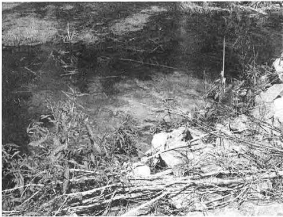
Photograph 1. Area of sediment deposit around small boil.
