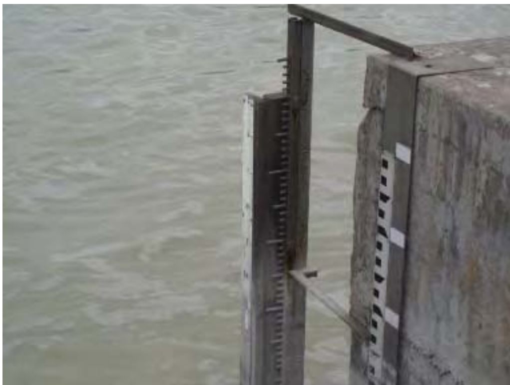
Photo No. 93: CADP - West embankment interior slope, close up of staff gage on intake structure.
