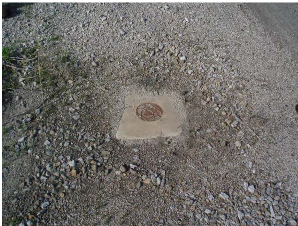
78. Piezometer PZ-2 on Pond D east embankment crest installed by BT 2 on 6/12/08.
