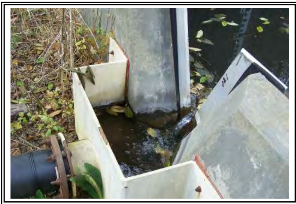
LLA v-notch monitoring weir for lower left abutment seepage.
