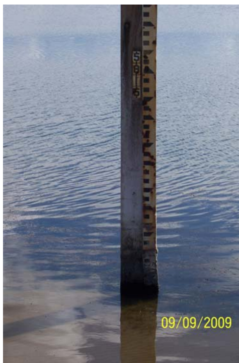
Photo 22: View of staff gage on upstream berm. Note lower markings difficult to read. Pond level at time of inspection was approximately 5810 feet.
