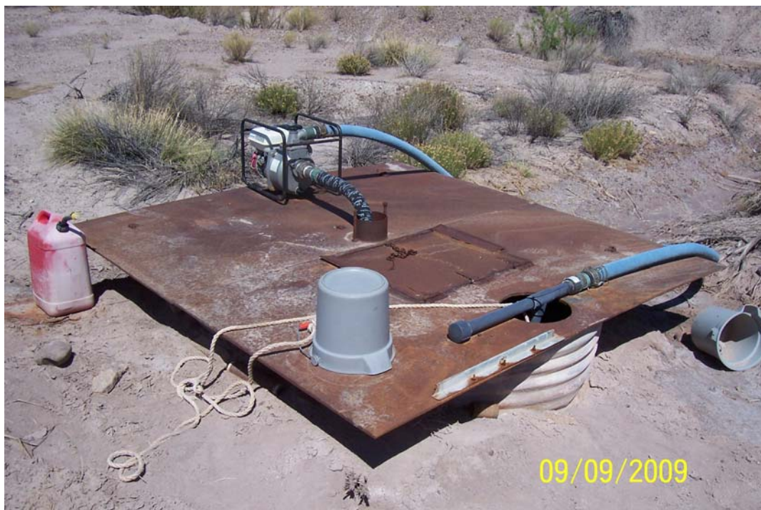
Photo 17: View of left toe drain sump, with gas pump, recirculation piping, and bucket used for flow measurement and seepage observations.
