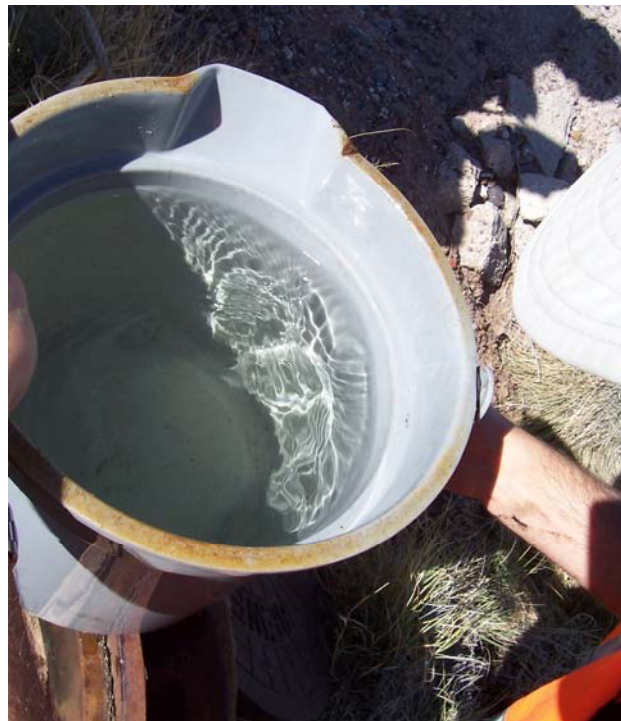
Photo 16: View of seepage water taken from left toe drain manhole.
