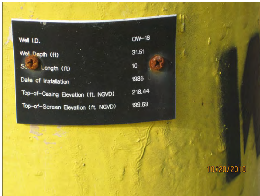
31 ASH POND 2-EXAMPLE OF OBSERVATION WELL IDENTIFICATION PLATE
