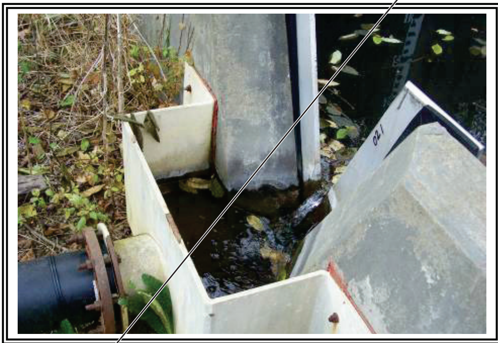
V-notch monitoring weir for lower left abutment seepage.
