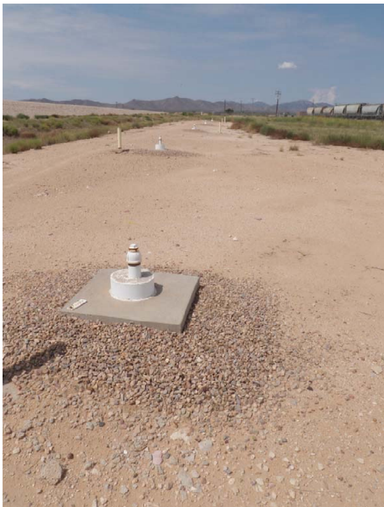
Photo 61: High precision survey monuments located in area where fissures were identified on north side of Scrubber Sludge Pond 2/ Evaporation Pond prior to construction. Note train on tracks located north of the facility.
