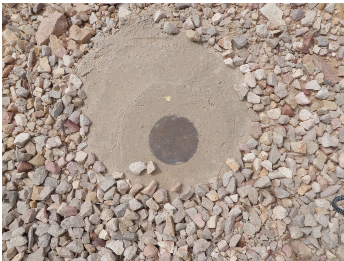
Photo 34: Survey Monument on crest of Ash Pond 2.
