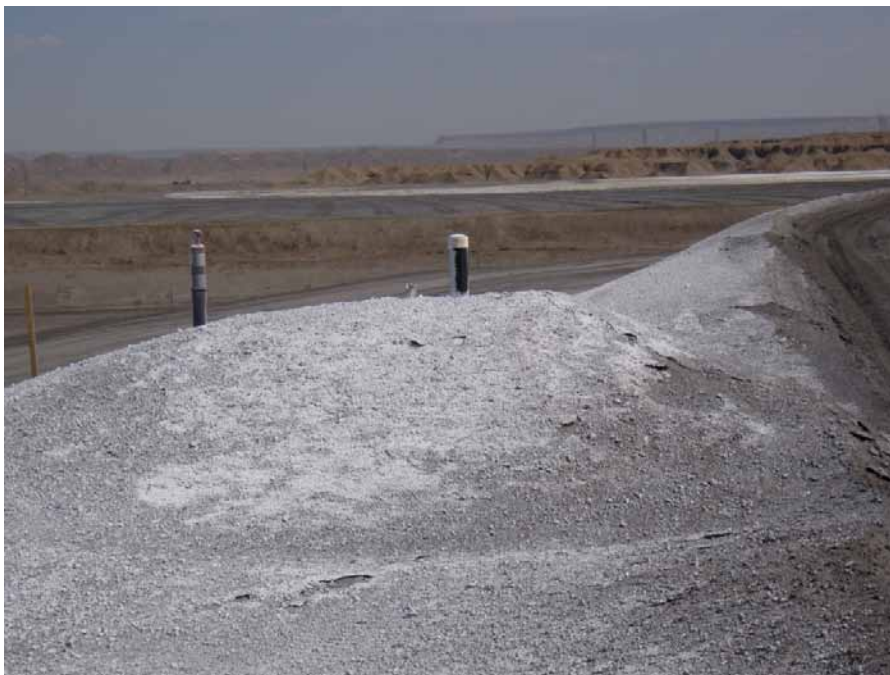
Photo 15 – LAI Instrumentation piezometers located on downstream crest of west dam near the decant drop inlet.
