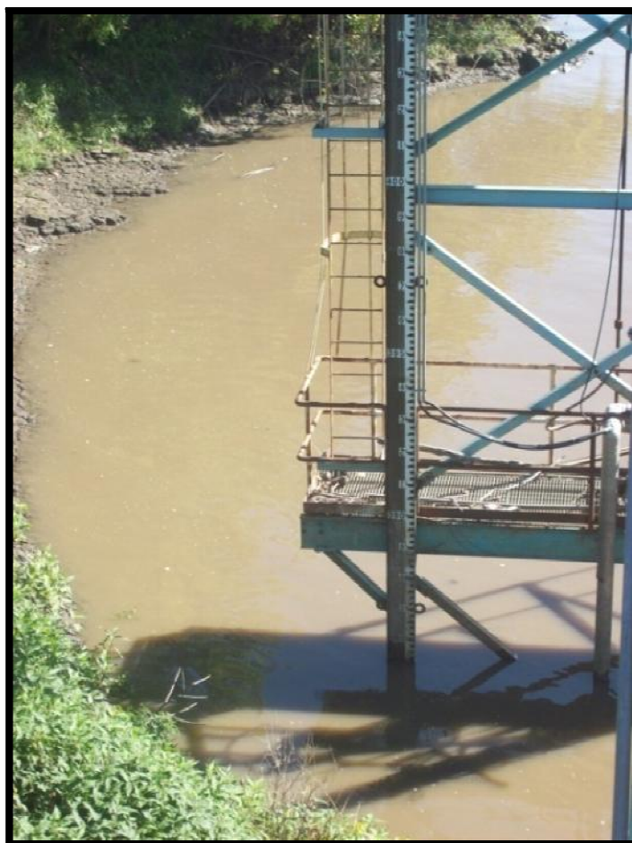
Figure 7: Staff gage at ash pond discharge area, Mississippi River. Outlet fully submerged.
