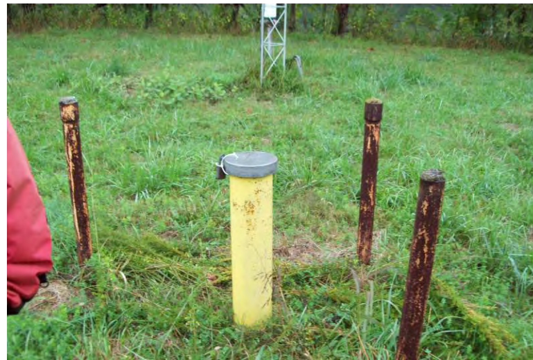
Photo 61: Monitoring well associated with coal pile storage at east embankment crest, looking east.
