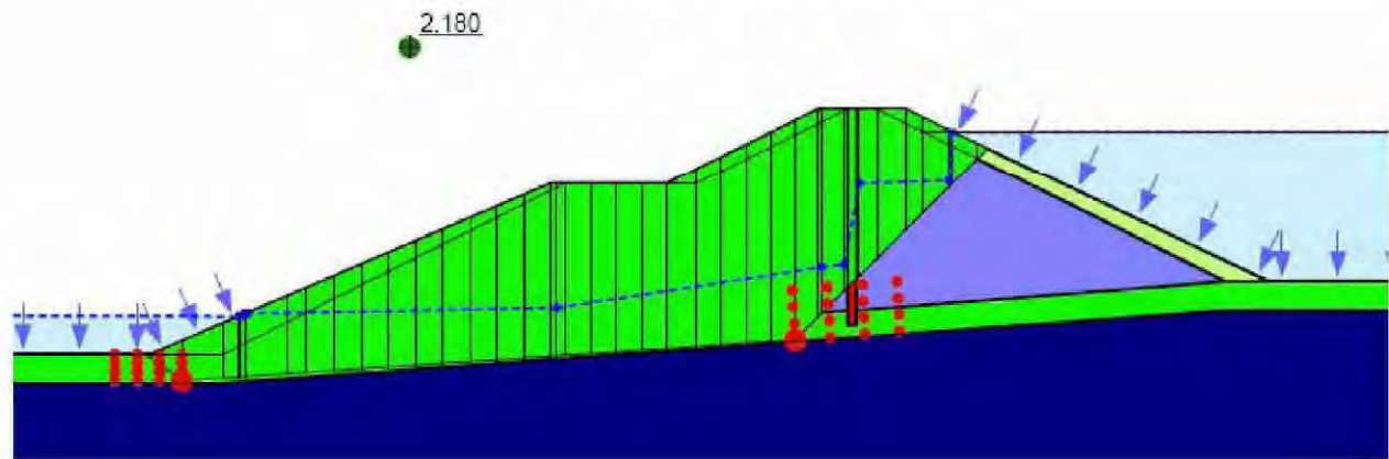
Figure 10A. Block failure of the dam and the associated safety factor under steady-state condition
