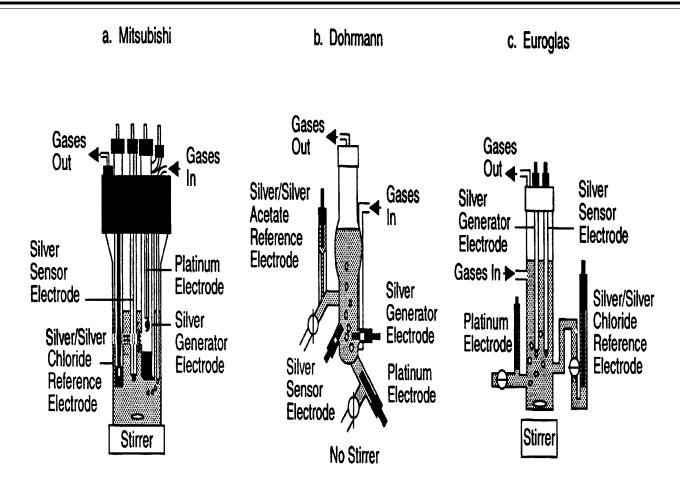
Figure 1. Microcoulometric Titration Cells (from Reference 7)
