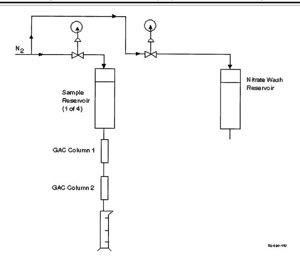
Figure 3. Schematic of the Column Adsorption System
