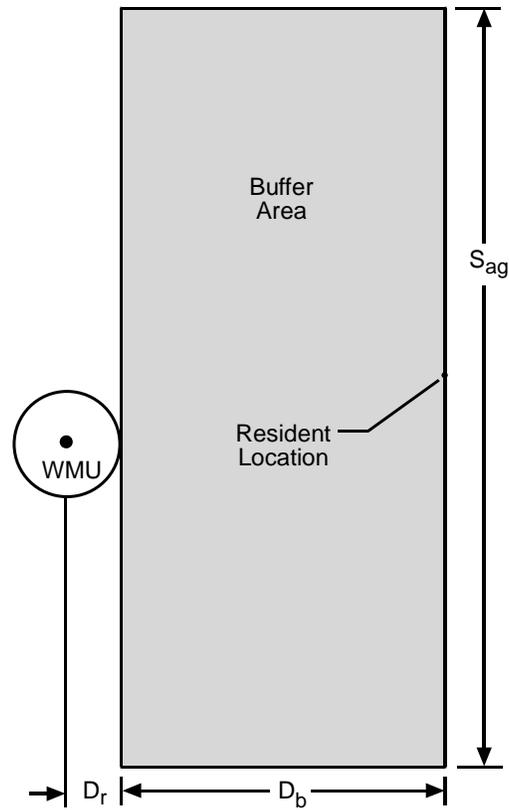
Figure 4-2. Conceptual site layout for residential aboveground scenario.
