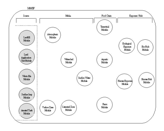
Figure 3.11 Graphical illustration of MMSP modules.
