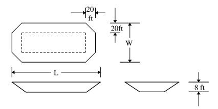
The number of wells (N) will be the half of the perimeter (P) of the waste management area, divided by 150 feet. That is, one well every 150 feet on the downgradient half of the perimeter of the 10 foot buffer zone surrounding the unit.
