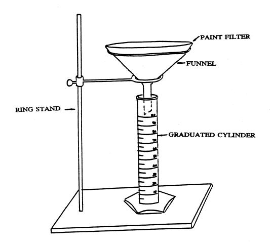
Figure 1. Paint filter test apparatus.
