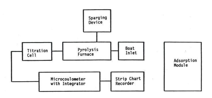
Figure 2. Flowchart of Analytical System
