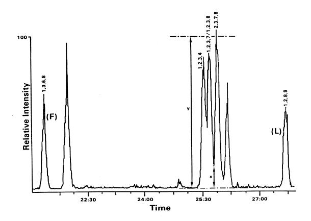
Selected ion current profile for m/z 322 (TCDDs) produced by MS analysis of GC performance check solution on a 60 m x 0.32 mm DB-5 fused silica capillary column with 0.25  $\mu m$  film thickness.
