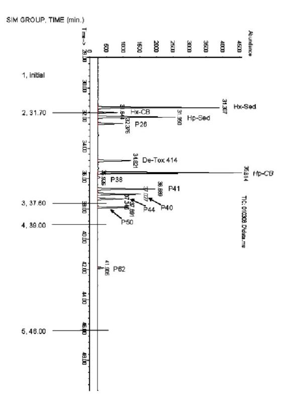
EXAMPLE GAS CHROMATOGRAM OF A FISH TISSUE EXTRACT WITH WEATHERED TOXAPHENE AND SPIKED USING DECACHLOROBIPHENYL
