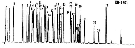
GC/ECD chromatogram of the PFB derivatives of phenolic compounds analyzed on a DB-5/DB-1701 fused-silica open-tubular column pair. The GC operating conditions were as follows: 30 m x 0.53 mm ID DB-5 (0.83  $\mu m$  film thickness) and 30 m x 0.53 mm ID DB-1701 (1.0  $\mu m$  film thickness) connected to an 8" injection tee (Supelco Inc.). Temperature program: 150°C (1 min hold) to 275°C (2 min hold) at 30°C/min.
