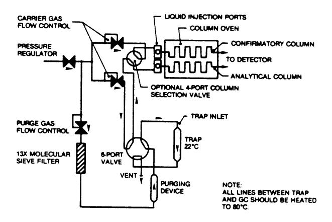
Figure 5 Purge-and-Trap System Desorb Mode For Method 8010, 8020, and 8030
