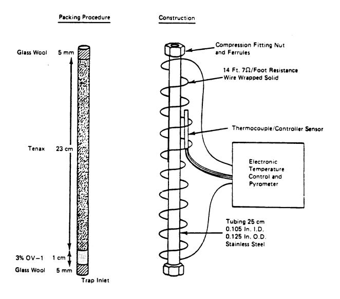
Figure 4 Purge-and-Trap System Purge-Sorb Mode For Method 8010, 8020, and 8030
