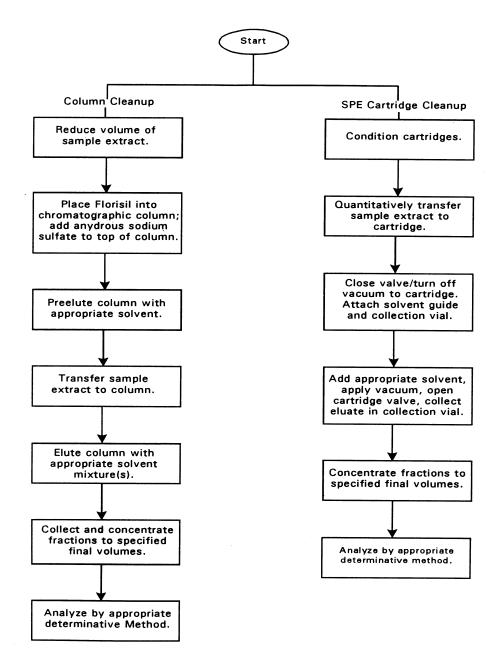
Note: Select specific procedures provided in the method depending on the type(s) of analytes of interest. See the method for details regarding the appropriate elution and collection procedures.
