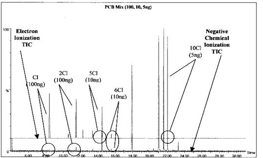
**Figure 2.** TICs of a Biphenyl Standard Mix using EI & NCI
