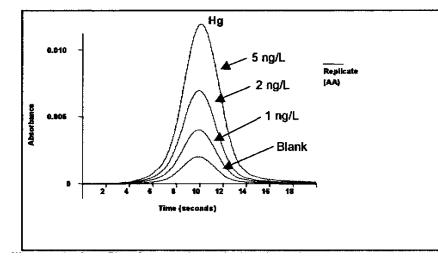
Amalgamation typically improves detection limits by a factor of ten. Bromate reagent acts more quickly than KMnO<sub>4</sub> and may be cleaner. This also can contribute to lower detection limits. The time of amalga- mation can be varied and increased times yield increased preconcentra- tion and lower detection limits. Figure 2 demonstrates peaks obtained from standards preconcentrated for 180 seconds, using 30 mL of solution.
