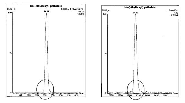
Figure 4. Both SIR and EIC yield a sufficient number of scans across the peak.
