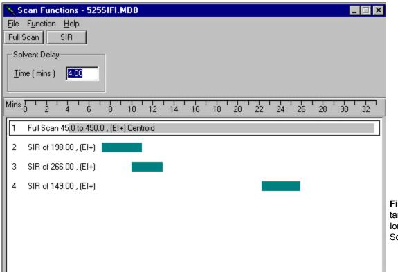
**Figure 1.** Simultaneous Selected lon and Full lon Scanning.
