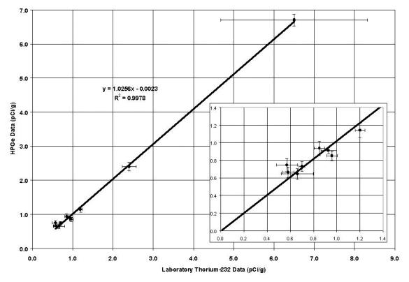
Figure 2. Correlation Between HPGe and Laboratory Data for Th-232 at a 31 cm Detector Height
