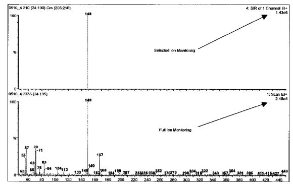
Figure 3. Spectra and signal intensity for bis-(ethylhexyl)phthalate using SIR and full scan mode.
