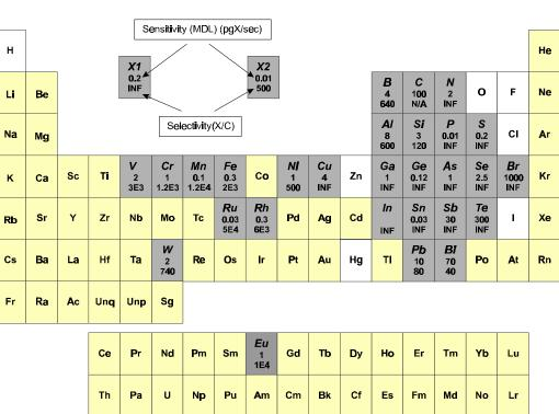
infinite selectivity: S, P, N, As, Se, Sn, Ge, Ga, Sb, Te, Br, Cu, In
