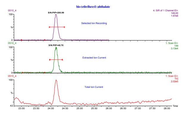
Figure 2. SIR and full scan signal-to-noise comparison.
