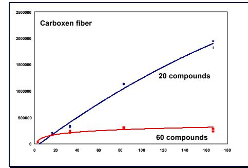
Linearity studies were conducted from 3.3 to 176 ppb with two test mixtures, one containing 60 compounds and the other containing 20 compounds. With the 60 compound standard, linearity flattens out as the concentrations increase. With the 20 component mixture, linearity is quite good for both compounds over the tested range. These results are consistent with the supposition that the fibers will saturate if too many components occur at these levels in the headspace.
