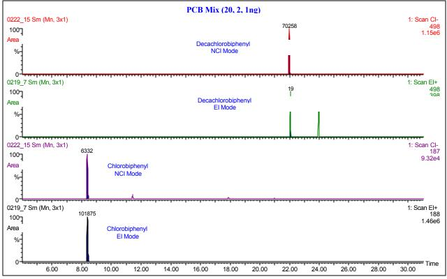
Figure 3. Monochlorinated and Decachlorinated biphenyls using EI & NCI.
