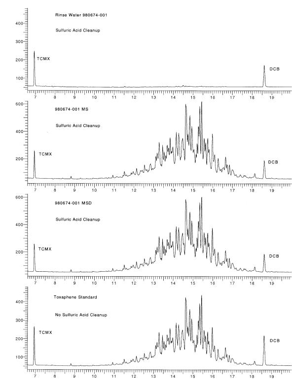
Figure 2. Comparison of Chromatograms of a Toxaphene Standard with Extracts of a Water Sample and Matrix Spike Samples
