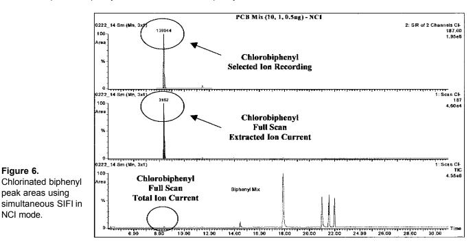
Additionally, simultaneous full ion and selective ion (SIFI) monitoring in one analysis can provide the ultimate combination of sensitivity and productivity. SIFI can be combined with either ionization technique, increasing sensitivity only where it is needed. It can extend the analytical range for analytes with widely disparate responses thereby eliminating many additional analyses.
