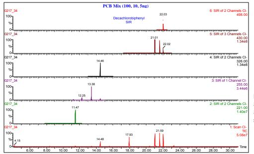
**Figure 5.** Simultaneous Selected Ion and Full Ion Scans for a biphenyl standard mixture.
