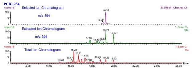
Figure 1. Aroclor 1254 acquired with NCI and simultaneous SIFI
