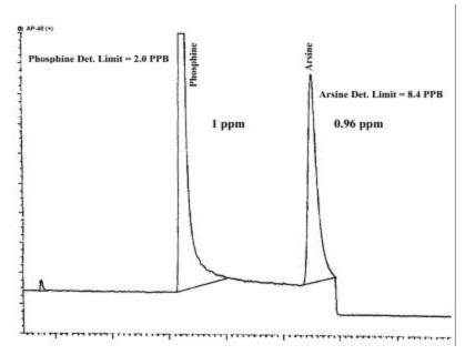
ing gases such as arsine. The PFPD can also simultaneously detect AsH3 and PH3 as shown in Figure 10 where propylene is the major component.
