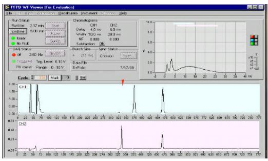
**Figure 12.** PFPD Data File Viewer Showing Phosphorus and Sulfur Chromatograms
