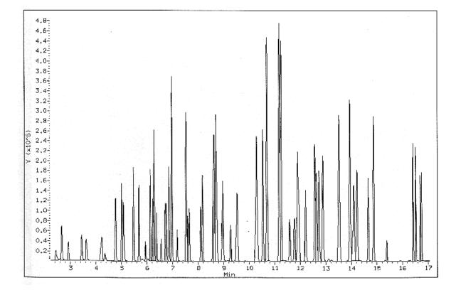
**Figure 2.** Total ion chromatogram of a 200 µg/L VOA calibration standard using a narrow bore capillary/direct interface system.
