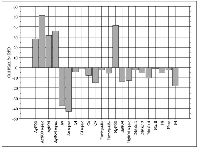
Figure. Bar chart of RPD of cyanide distillation recoveries from experiments without and with added magnesium chloride.
