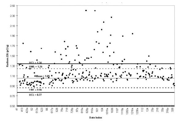
Figure 4. Control Chart for Radium-226 (Dry Wt. Basis)
