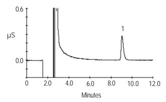
thiocyanate display any significant retention on either column using the elution conditions described above. Perchlorate is resolved by at least 2 minutes from the nearest eluting anion, thiocyanate, which would not be typically found at high levels in drinking or ground waters.
