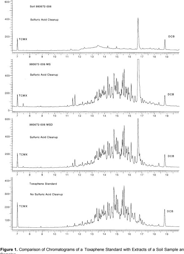
Figure 1. Comparison of Chromatograms of a Toxaphene Standard with Extracts of a Soil Sample and Matrix Spike Samples
