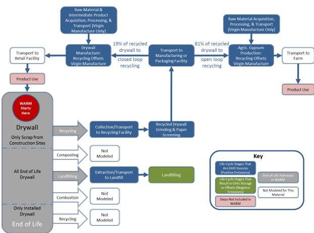
Drywall, also known as wallboard, gypsum board or plaster board, is manufactured from gypsum plaster and a paper covering. Exhibit 2 presents the sources of drywall entering the waste stream.
