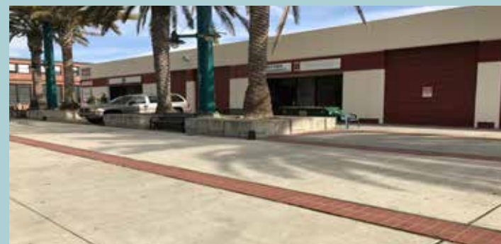
Figure 9. Industrial and commercial uses front onto Park Avenue in Emeryville, CA. The shared street is curbless and uses brick pavers to demark a narrowed drive aisle and parking areas. Raised planters with palms and landscaping define parking, seating, and pedestrian priority spaces.
