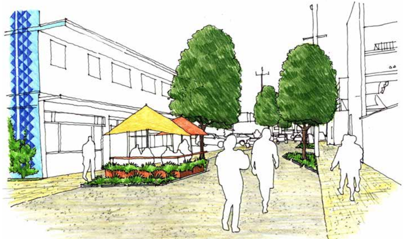
Figure 14. Long-term perspective. Parklets, permeable paving across the street's full width, and landscaped or stormwater planters with street trees, add greenery, shade, and improve stormwater quality. Parklets and planters can assist in creating curves (chicanes) that slow down traffic and create social spaces along both sides of the street.
