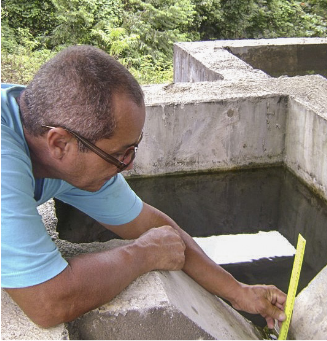
Measuring flow changes in the inlet to an experimental slow sand filter being adapted for the Mulas community in Patillas, Puerto Rico. Photo credit: Center for Environmental Education, Conservation and Research, Inter-American University of Puerto Rico.
