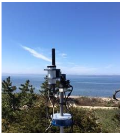
EPA scientists are using spectrometers to measure compounds which form ozone to better understand the underlying causes of high ozone across the Long Island Sound Region.
