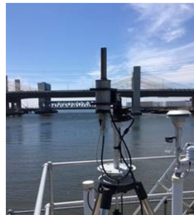
EPA scientists are using spectrometers to measure compounds which form ozone to better understand the underlying causes of high ozone across the Long Island Sound Region.
