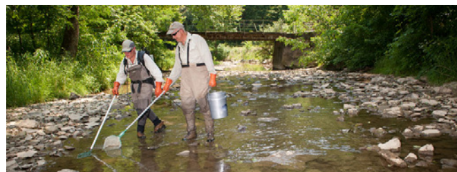
Using electric current to stun fish during a stream survey. Photo credit: U.S. Environmental Protection Agency.
