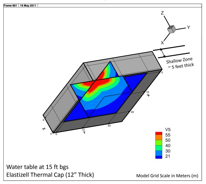
Simulation – 03D.i: 20% Steam (60C) at 50 scfm – 100 Days Shallow Soil Zone – Temperature Distribution
