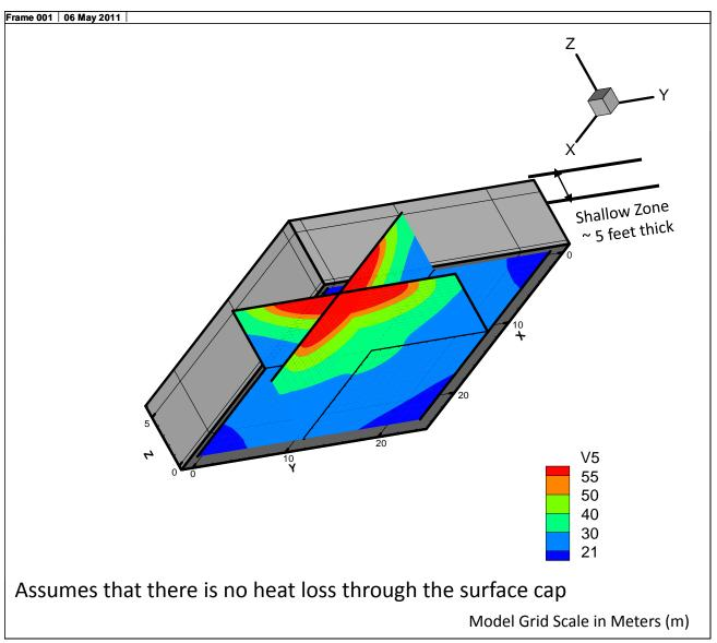
Simulation – 03A: 20% Steam (60C) at 50 scfm – 10 Days Shallow Soil Zone – Temperature Distribution
