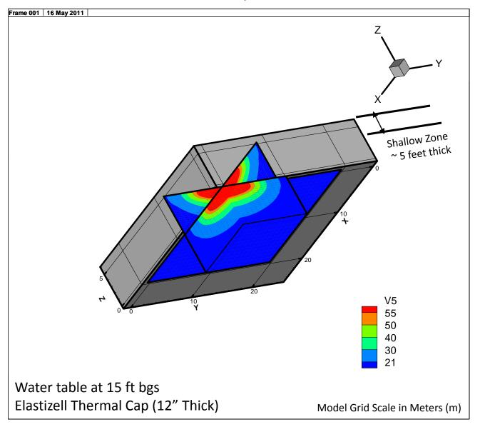
Simulation – 03C: 20% Steam (60C) at 50 scfm – 50 Days Shallow Soil Zone – Temperature Distribution
