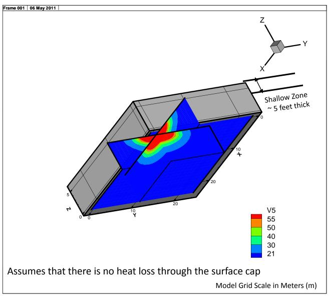
Simulation – 02B: 20% Steam (60C) at 50 scfm – No Surface Heat Loss – 50 Days Shallow Soil Zone – Temperature Distribution
