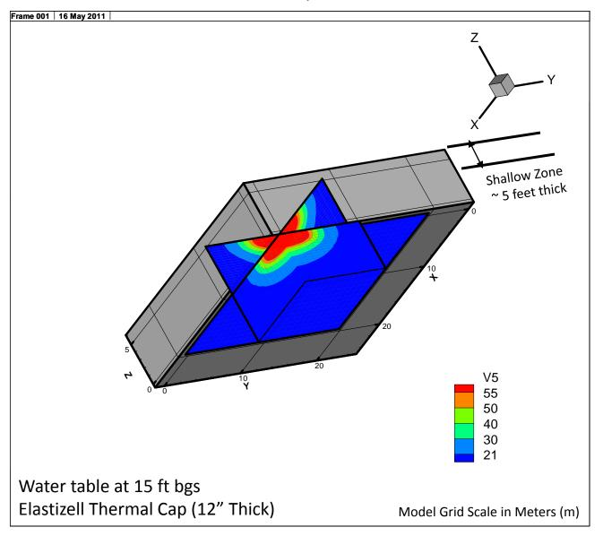
Simulation – 03B: 20% Steam (60C) at 50 scfm – 20 Days Shallow Soil Zone – Temperature Distribution
