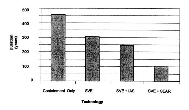
Figure 7-5 Projected Durations from Present to 5  $\mu$ g/L Benzene, versus Technology
