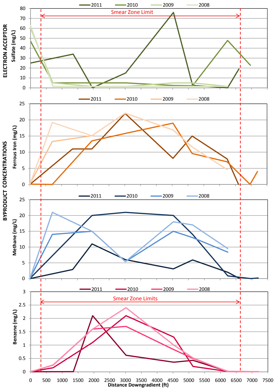
FIGURE 4-16. DISSOLVED PHASE BENZENE AND HYDROGEOCHEMICAL SUMMARY VERSUS DISTANCE FIVE-YEAR GROUNDWATER CORRECTIVE MEASURES IMPLEMENTATION REVIEW CHEVRON CINCINNATI FACILITY, HOOVEN, OHIO
