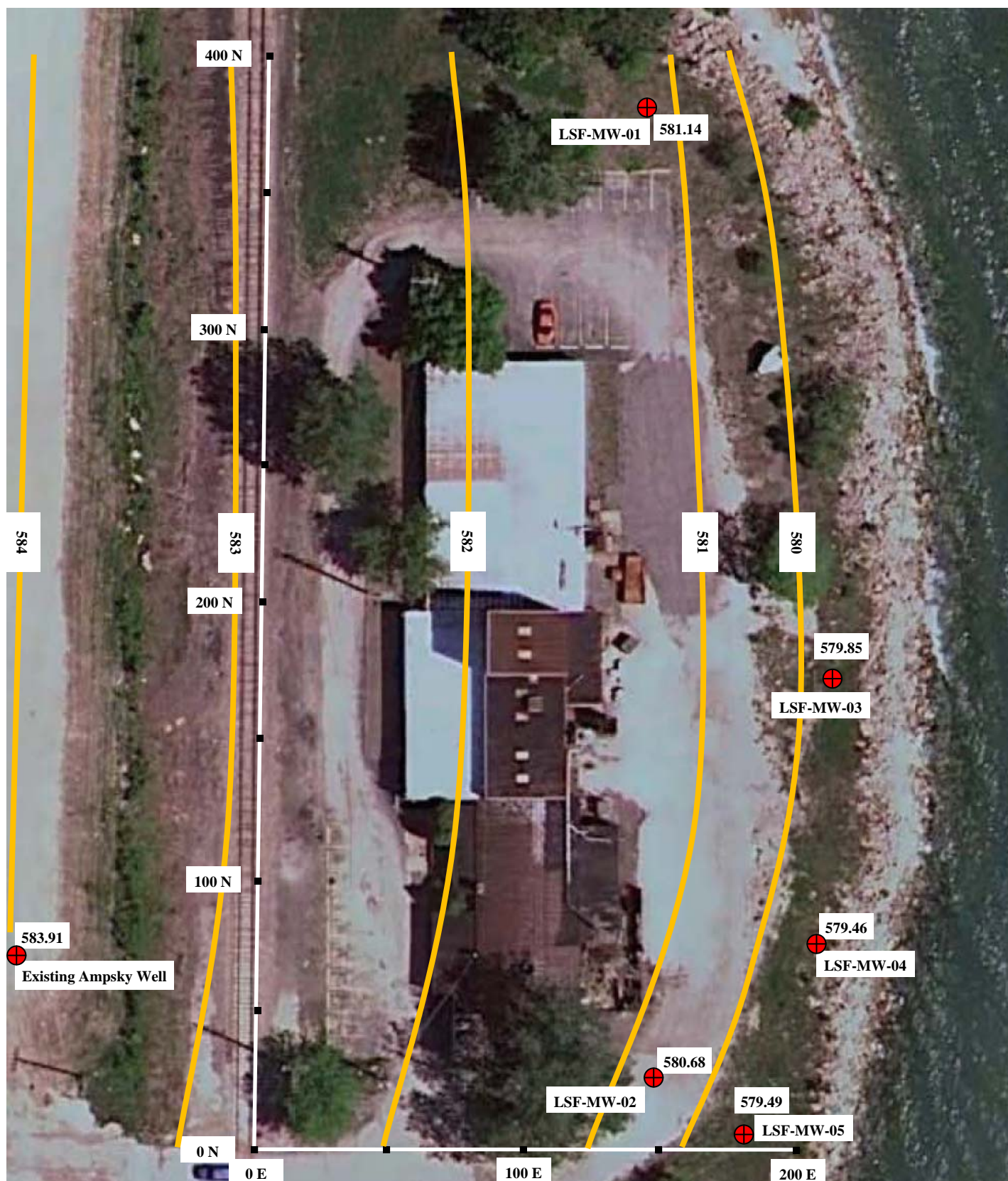
Figure 3 Groundwater Sample Locations and Groundwater Elevations, January 18, 2012 Former Lake Shore Foundry Waukegan, IL 60085
