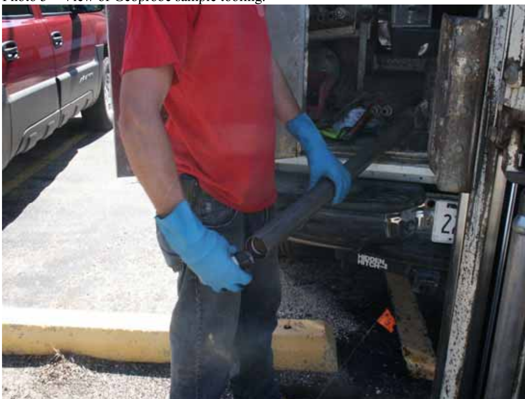
Photo 4 – View of Geoprobe sample tooling, removal of soil sample.
