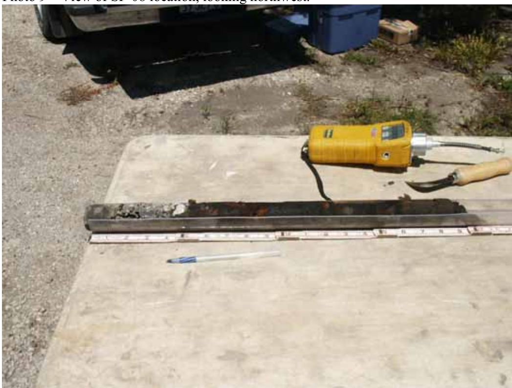
Photo 10 – View of soil sample and MinnieRae 2000 PID instrument.
