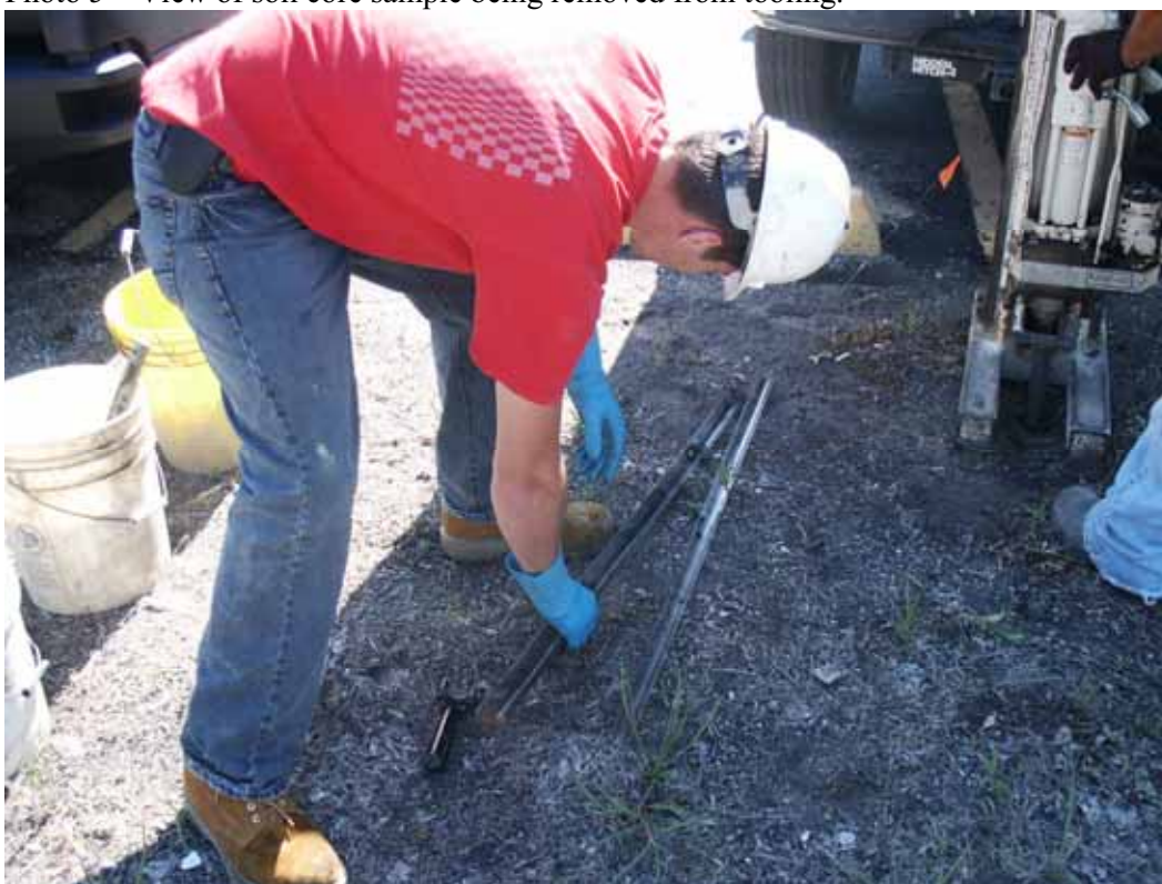
Photo 6 – View of soil sample being opened within acetate tube liner.
