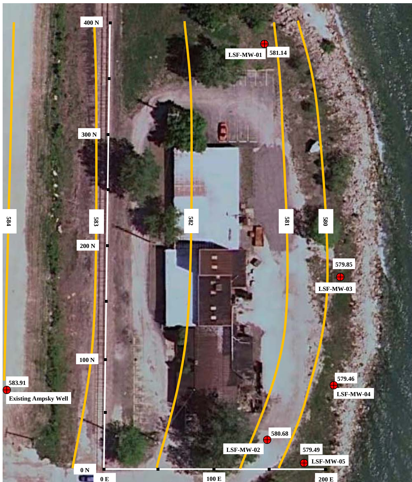
Figure 1 Groundwater Sample Locations and Groundwater Elevations, January 18, 2012 Former Lake Shore Foundry 653 S. Market St. Waukegan, IL 60085
