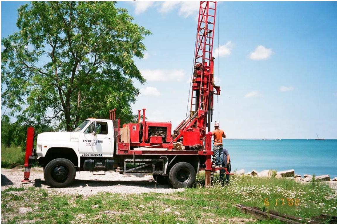
Photo 1 – View of drilling methods with hollow stem augurs at LSF-MW-03.
