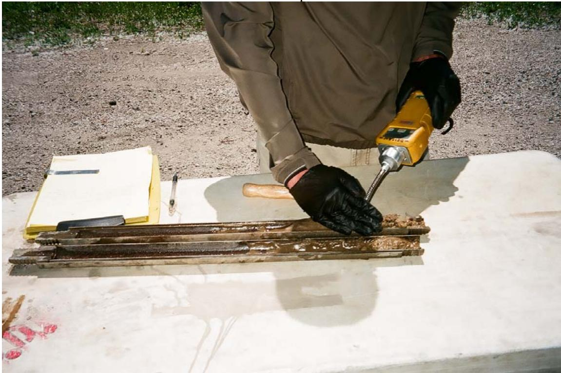
Photo 6 – View of soil sample field screening with Minnie Rae 2000 PID.
