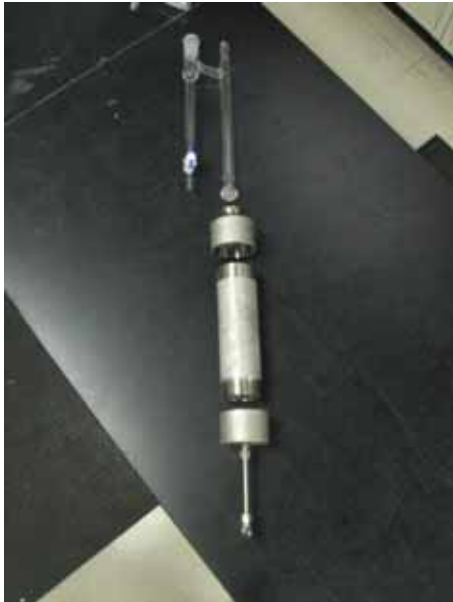
Figure 1 Stainless Steel Pipe, Caps, and Dean-Stark Glassware.
